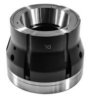
Check the concentricity and face runout of the spindle adapter before mounting the collet seat assembly. Neither should exceed .0002" ( $5\mu m$ ). If the indicator reading is more than .0002" ( $5\mu m$ ), remove the spindle adapter and clean the surfaces again before remounting.
